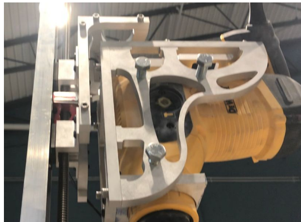
Figure 8: Side View of Drill Mount - Showing Lead Screw Connection
